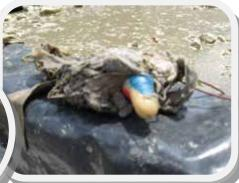
A section of pipe plugged with grease. The hole is from the auger when they tried to clear the blockage.
